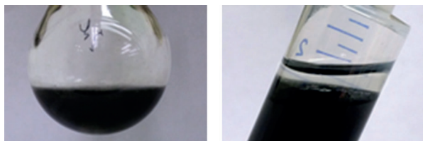
Figure 2. Appearance of a reaction mixture during the semihydrogenation process (left) and upon extraction with ether (right).
